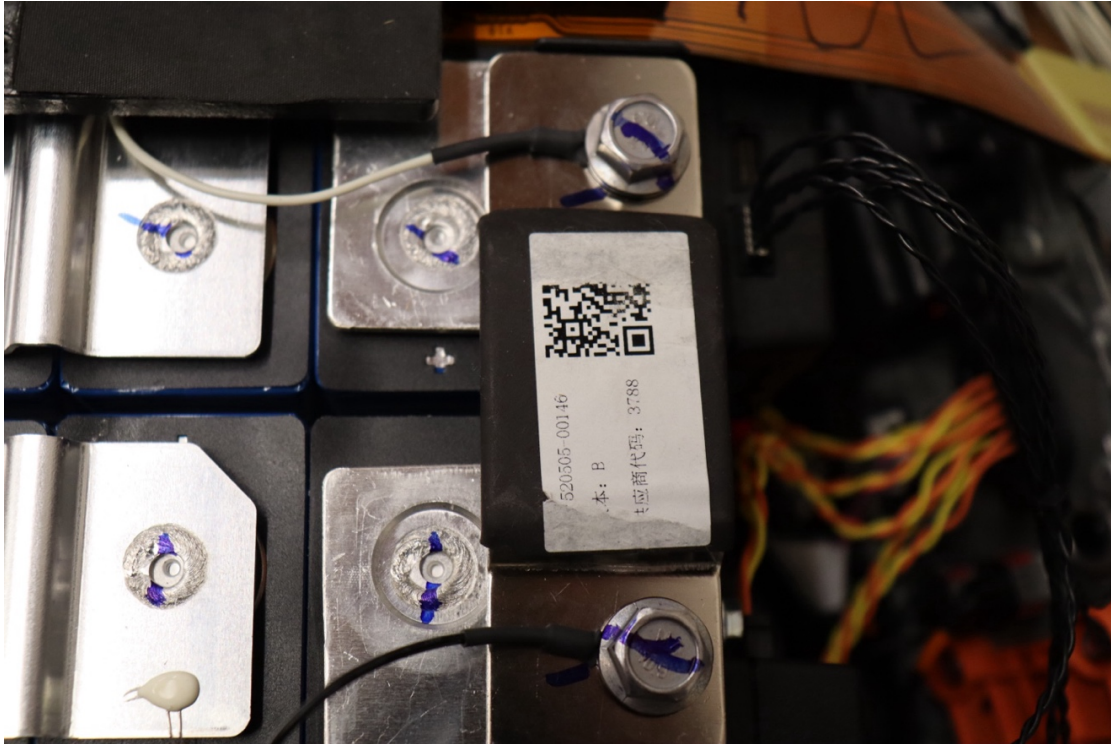
19) Optional ring terminal connection of LTC A1, W18 (white) and LTCA2, W0 (black)
