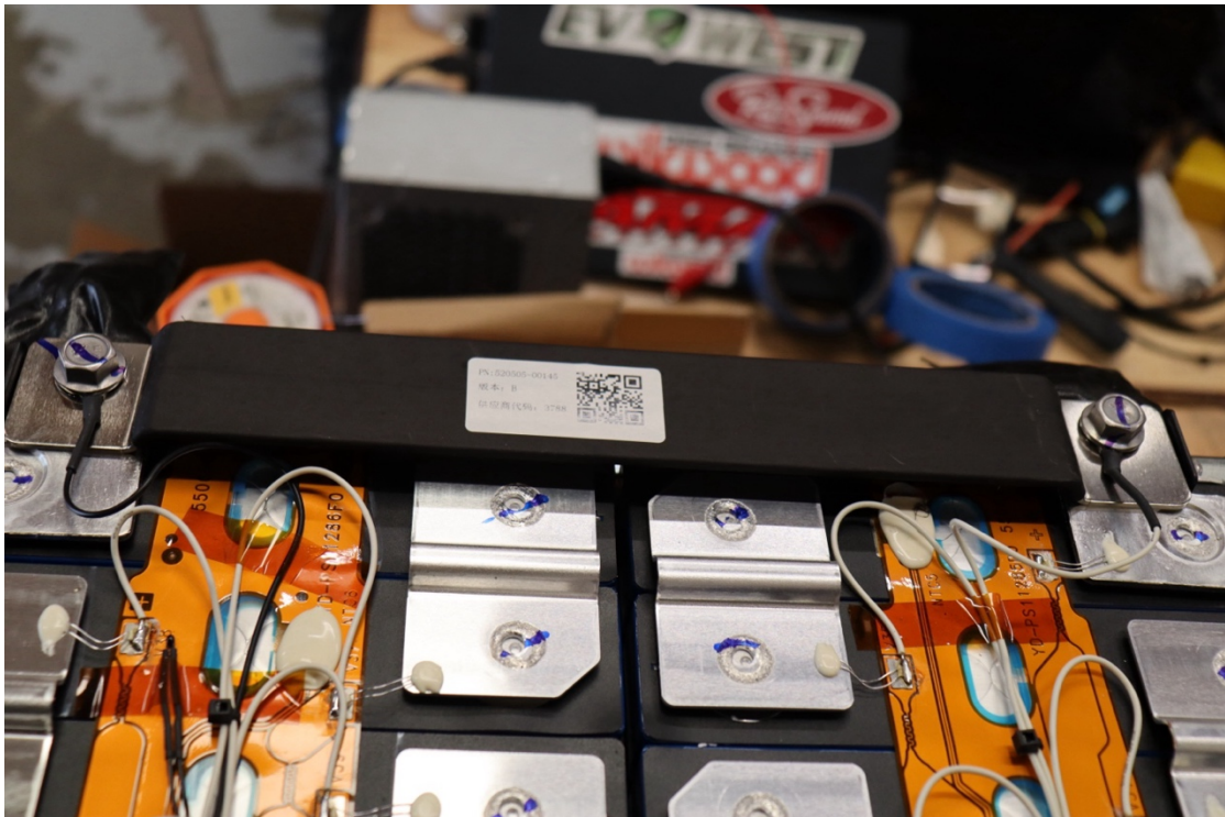
23) LTC A3, W0 (left side black wire) LTC A2, W18 (right side white wire)
