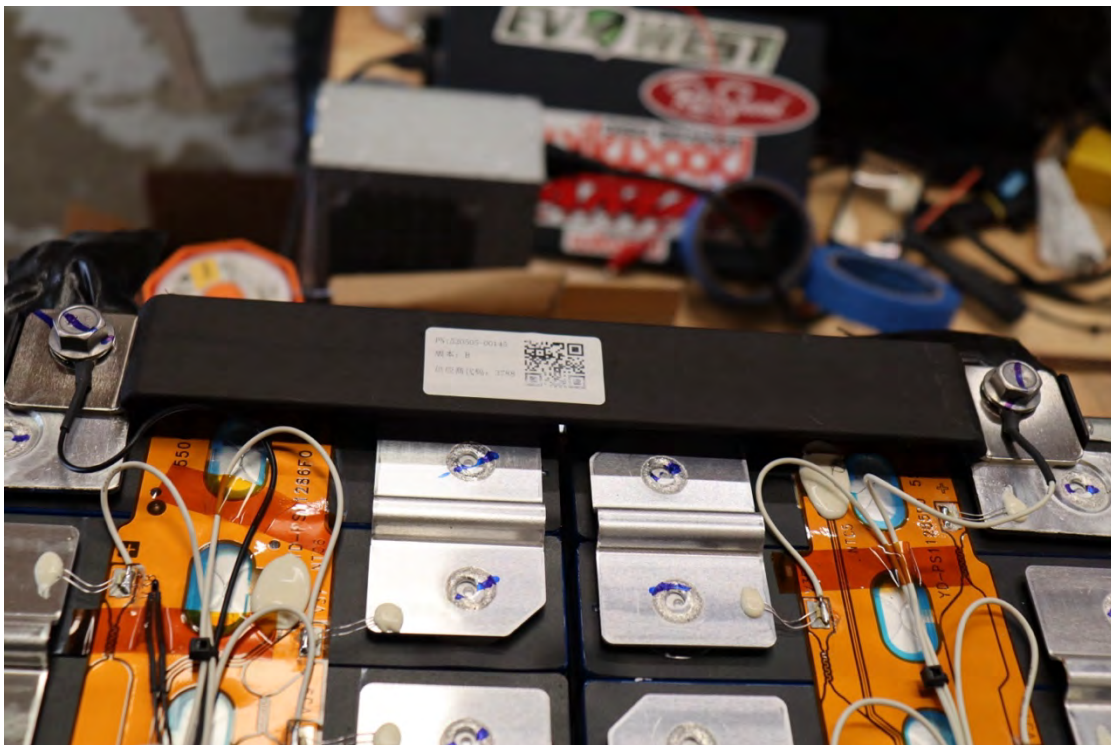
22) LTC A3, W0 (left side black wire) LTC A2, W18 (right side white wire)
