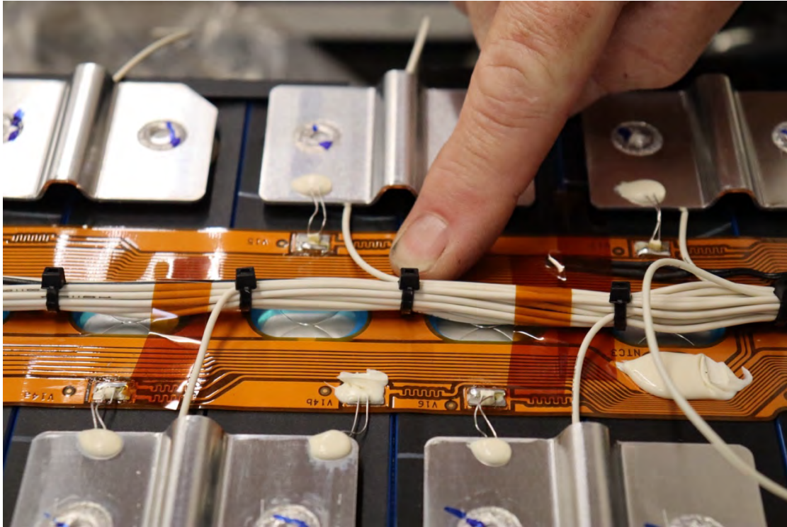
12) Secure harness wire bundles with zip ties. One at each all seam
