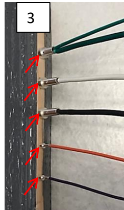
Insert wires into pins. They should push in by hand but be very tight. Weep hole faces up.
