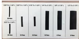
Heat shrink assortment sizes 5/32" to 3/4" Dry locations – standard Wet locations – adhesive lined
