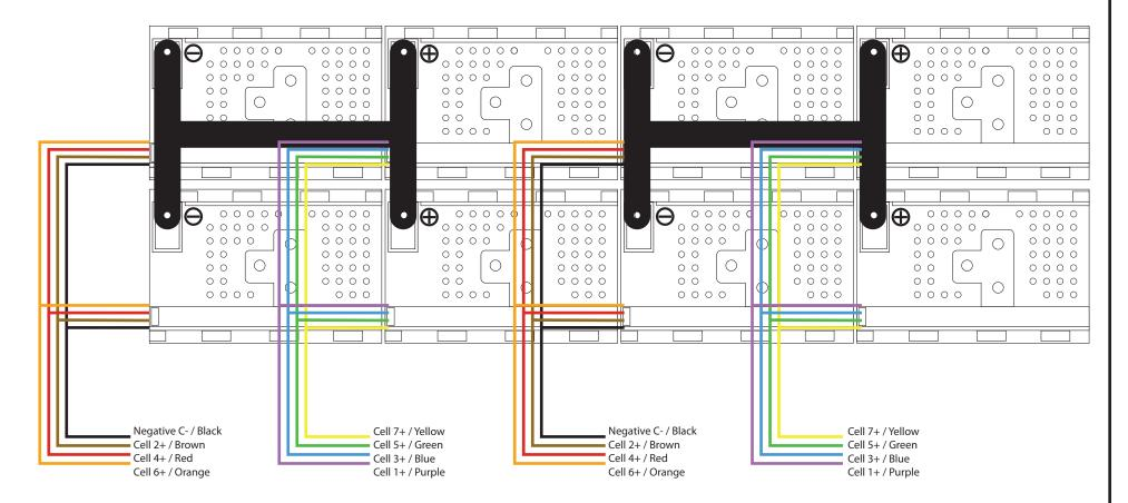
Note: By combining the BMS cell leads for the two cells in parallel, both of these modules can now be monitored as one in the BMS system, and the connection allows capacity balancing between the two modules at the cell level.
