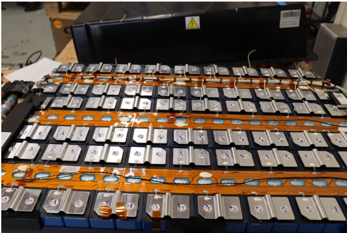
14) Trim wires to desired lengths
