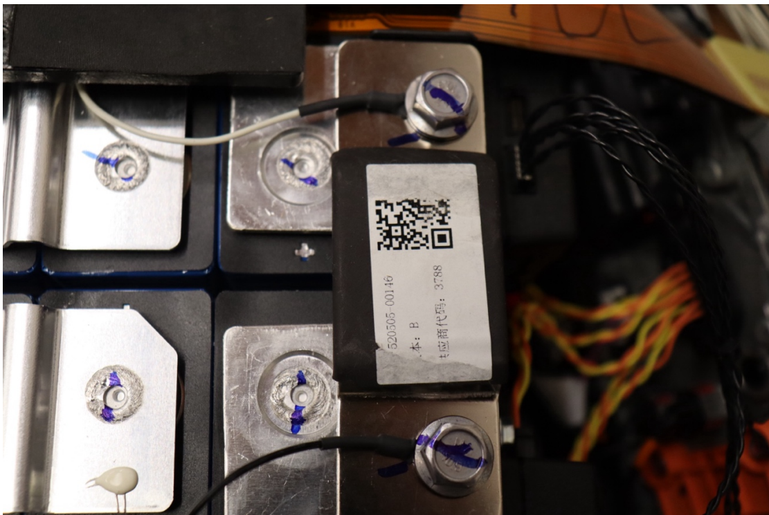
19) Optional ring terminal connection of LTC A1, W18 and LTCA2, W0 and LTCA2, W18
