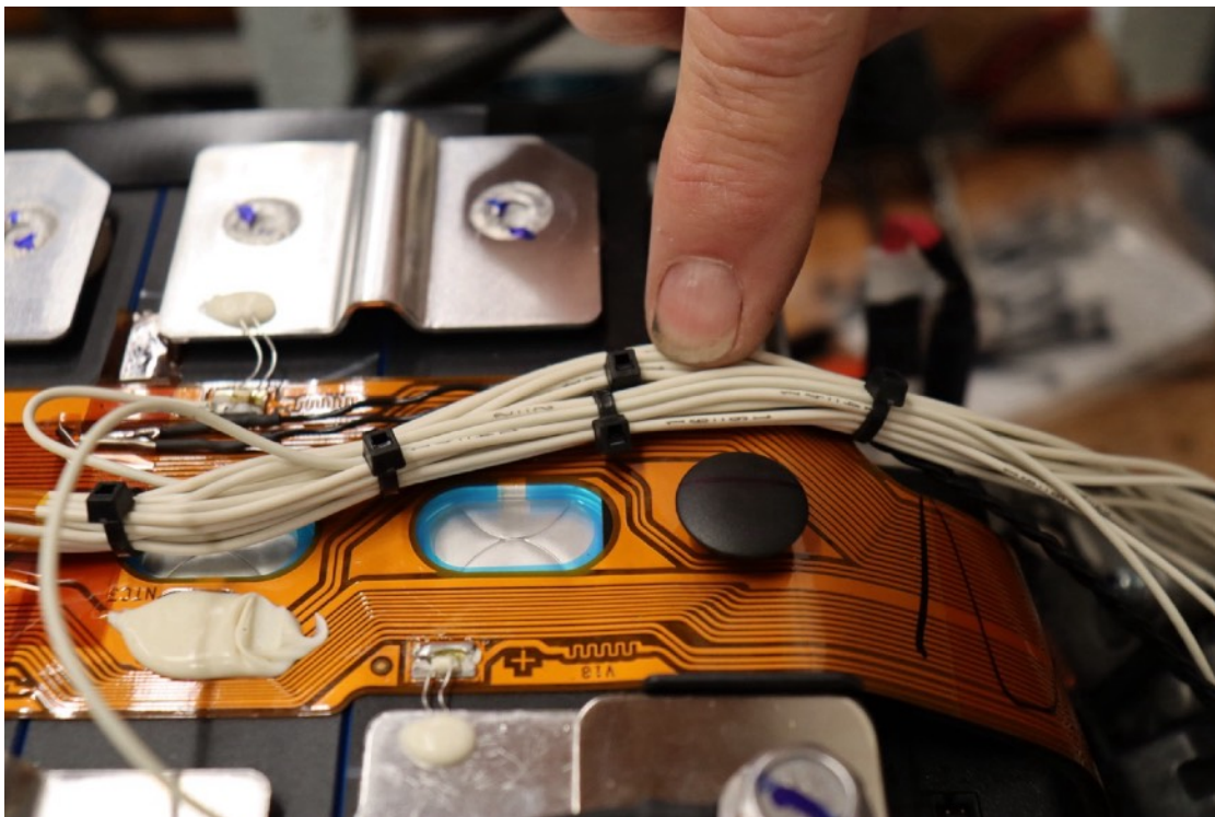
17) Solder wires to cell tap pads on ribbon cable
