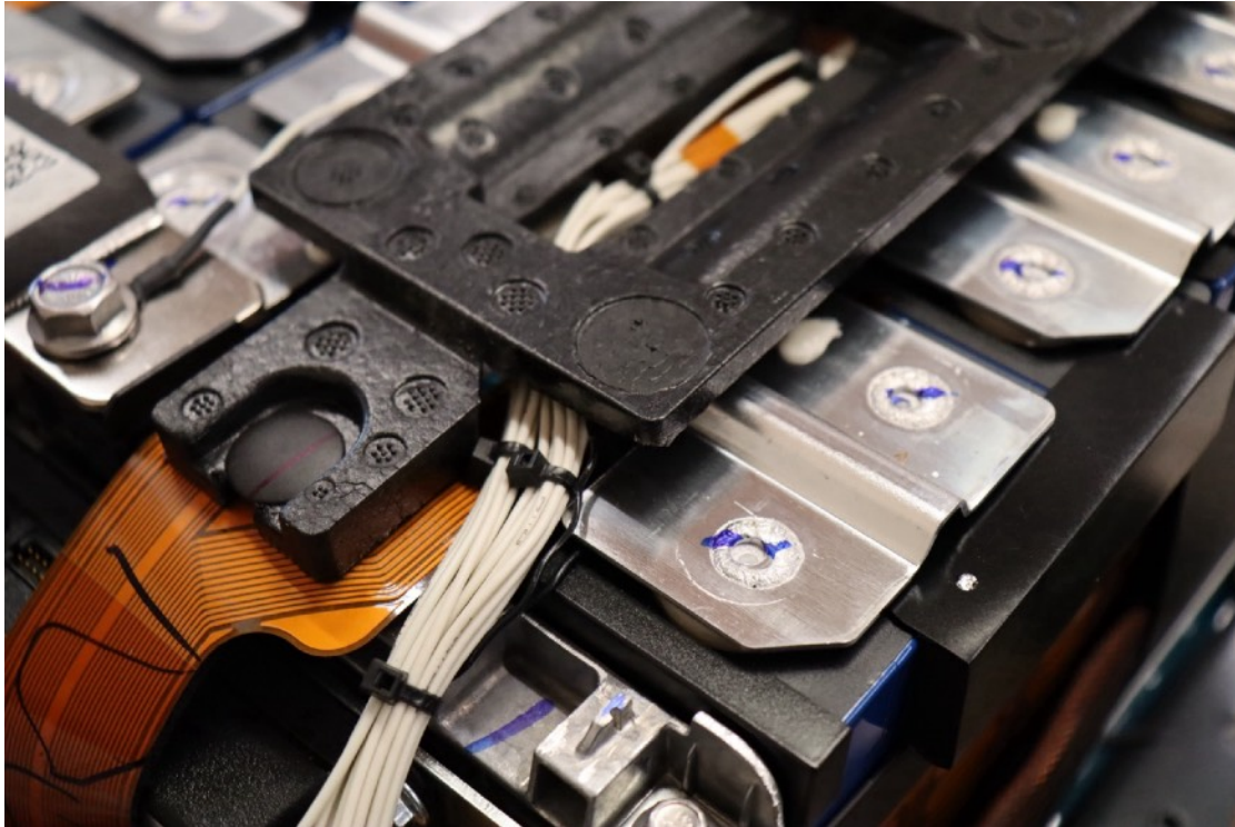
18) Route wire bundle to side of foam retainer pin for clearance exiting pack
